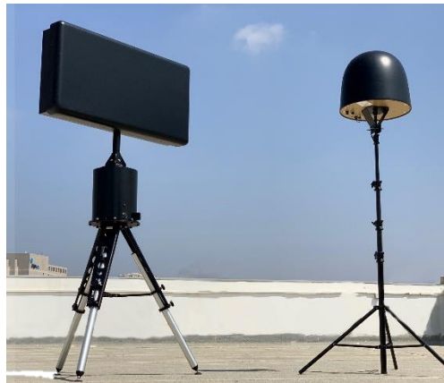
Detection system including Radar+ DF
